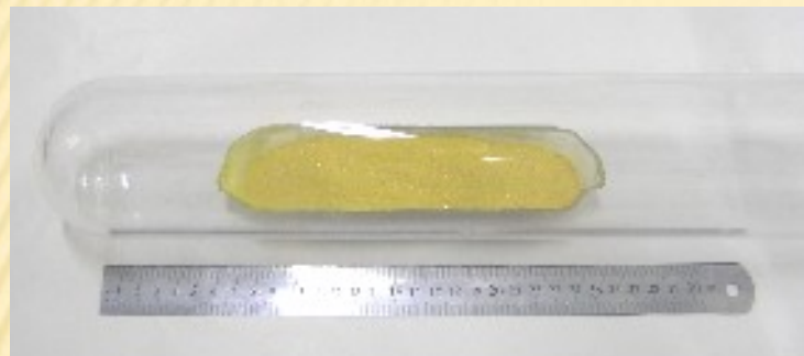
\text{Zn} + \text{Se} = \text{ZnSe} Synthesis at 1200 K in inert atmosphere
