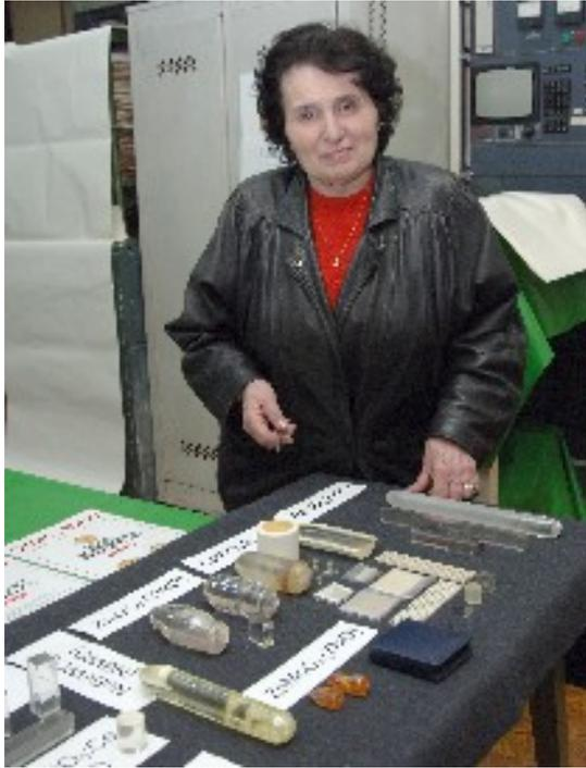
For the first time,  $\text{PbWO}_4$  scintillation crystal had been developed by us for studies in the field of high energies. Possible applications of this crystal include studies of double beta-decay, searches for dark matter and its use as anticoincidence shield and active light-guide
