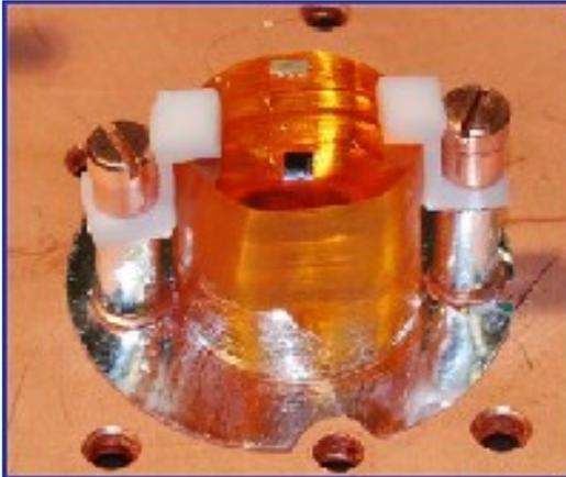
$\text{ZnMoO}_4$  crystal mounted on copper cryostat.
